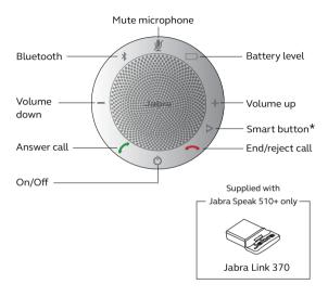
\*Newer Speak 510 variants (with the Smart button) have a Ver. ID beginning with D, or later. Older Speak 510 variants (without the Smart button) have a Ver. ID beginning with A, B, or C.
