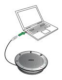
Plug the Jabra Speak 510 USB cable into any available USB port on your computer to charge the battery. The battery light is red when charging, and green for 1 minute when fully charged.
