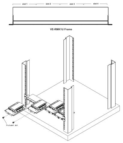
Note: Up to 4 Secure Device Servers can be secured onto a VE-RMK1U frame.
