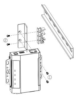
3. Hang the unit onto the DIN rail.
