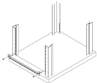
4. Align the device and mounting plate assembly to one of the slots on the VE-RMK1U frame, and then secure the mounting plate to the frame with the plastic captive screw provided.
