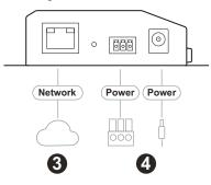
5. After supplying power, wait for about 50 seconds for the Secure Device Server to be ready and lights its status LED in constant green.
