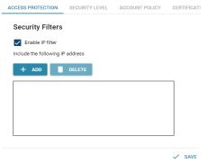
To enable exclusive access only for certain IP address(es), check **Enable IP** filter, and click the **ADD** button to add the desired IP address(es).
